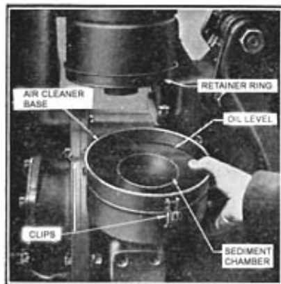
Figure 11 Cylindrical Type Air Cleaner
