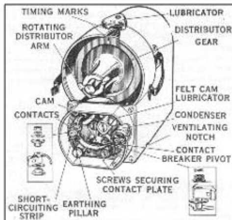
Figure 22 Stationary Type Contact Breaker Adjustment
