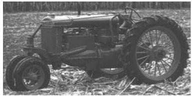
Fordson All-Around (a.k.a. Fordson Row Crop in U.S.) Modest revision of the Fordson N with tricycle style wheel arrangement Produced beginning in 1937 at Dagenham
