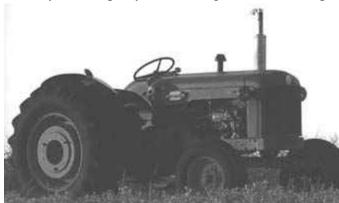
**Fordson Power Major** Featured a more powerful engine Diesel, gas, and distillate versions available Produced from 1958-1961 at Dagenham
