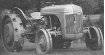
Ford 2N (a.k.a. Ford-Ferguson 2N) Featured steel wheels Generator and battery of 9N replaced by magneto All other specifications similar to Ford 9N Produced from 1942-1947 at Dearborn, Michigan
